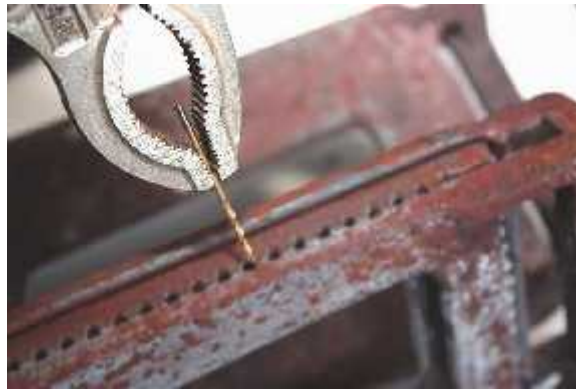
Use 1/16 drill bit to ream gas port
