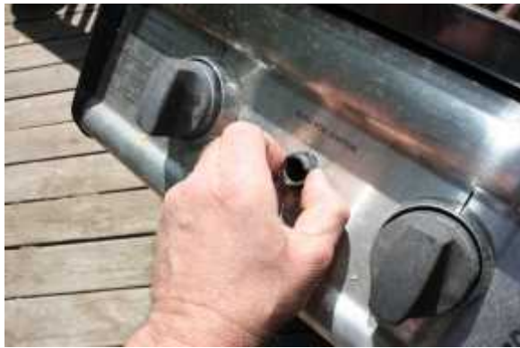
To remove igniter, unscrew the nut on the control. HANG ON TO THE NUT!!!
