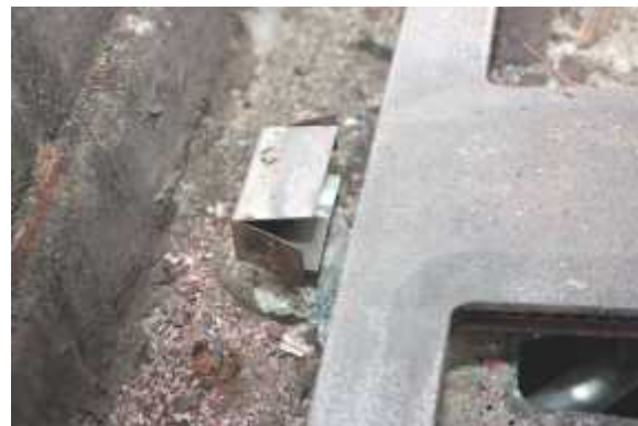
This is an electrode-collector box from a Great Outdoors 1000 grill. This box bolts onto the grill bottom.
