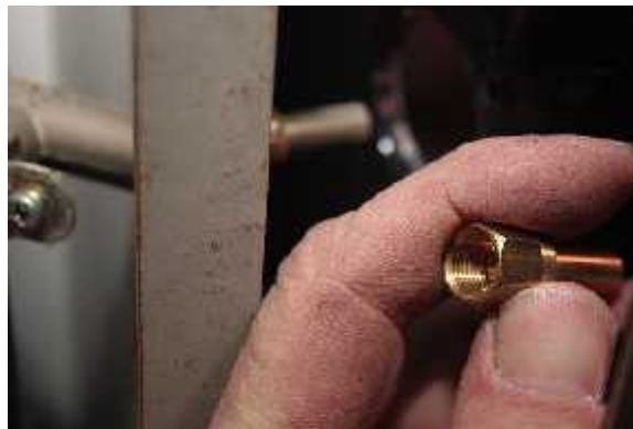
Check and clean 3 main burner orifices, one side burner orifice and the infrared burner orifice.
