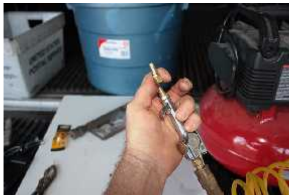
Clean and blow out each orifice with compressed air
