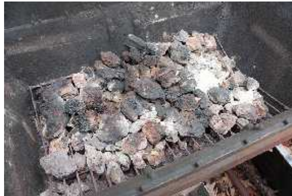
My old, caved in, Falcon rock grate. Note where it has caved in. It needs replacement.
