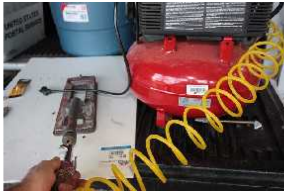
Use air hose to blow out burner-inside and outside. Canned air, used for dusting keyboards, works but not as well.
