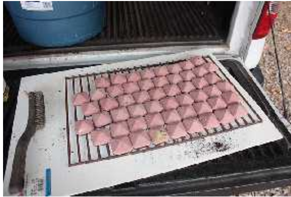
Great Outdoors 1000 Rock Grate with Rock (ceramic), while used, is still in “usable” condition.
