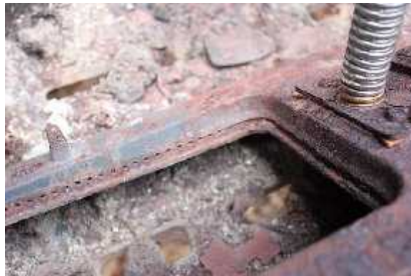
My Falcon burner could be brushed down and the gas ports reamed with drill bit. Then it should be blown out with compressed air. It isn't worth it to me.
