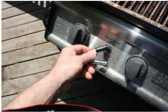
Check igniter. New battery should “click” if it is good.
