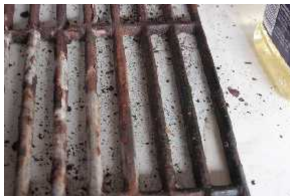
Cast iron grids (from Great Outdoors DG450) - wire brush and wipe with vegetable oil. Oil the grids on both sides between uses to reduce rusting.
