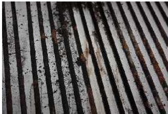
Porcelain coated grids (steel rod) showing brushed down area which was oiled with vegetable oil.
