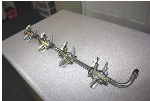
This is a valve assembly from Capt'n Cook with "flame thrower" igniters. These igniters are clamped to a pipe manifold.
