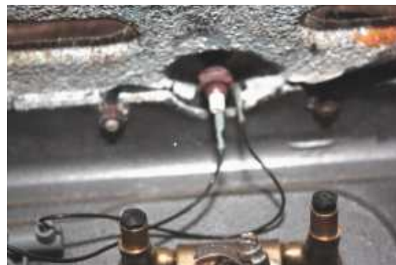
This is an electrode-collector box from a Great Outdoors 1000 grill. This box bolts onto the grill bottom.
