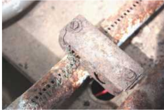
This is an old "clamp on" electrode-collector box from a Ducane 5004SHNE
