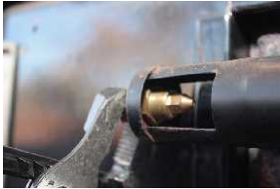
Loosen nut holding orifice fitting to venturi opening.
