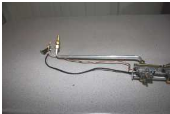
This is a valve assembly from an old post mounted valve gas grill. The manifold is the center piece that attaches to the post and receives the gas supply. The orifices are located in the valve ends that the burner venturi tubes slide over.
