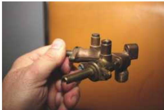
This is a valve assembly from an old post mounted valve gas grill. The manifold is the center piece that attaches to the post and receives the gas supply. The orifices are located in the valve ends that the burner venturi tubes slide over.
