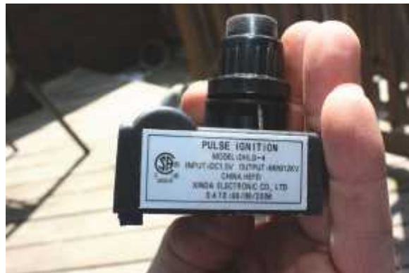
It's easier to hook up the wires before you put the igniter back in.
