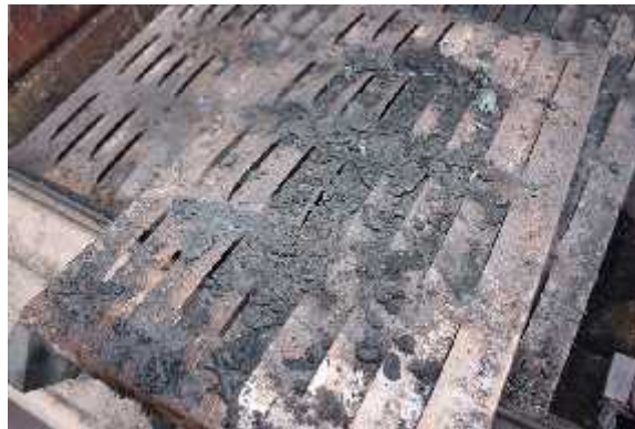
Remove and clean Heat Plates
