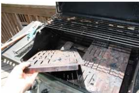
Remove the grids, heat plates and burners to get to the electrode.
