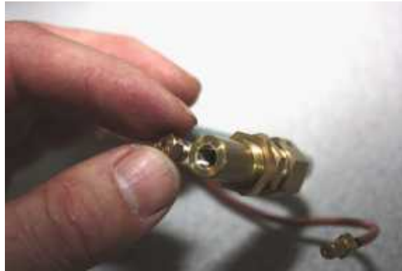
This is an orifice removed from a valve extension fitting.
