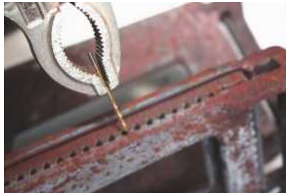
Cleaned (reamed) gas ports using a 1/16 drill bit.
