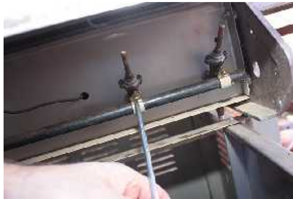
To replace the valve, remove the screws holding the valve to the manifold. CHECK FOR LEAKS AND TEST before using the grill.
