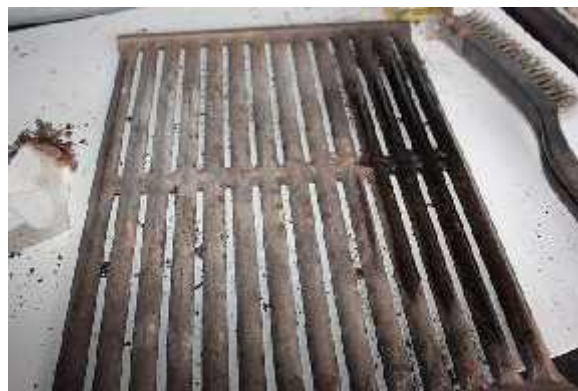
Ducane stainless, stamped steel grids showing rust which is possible even with the best (304 grade) stainless steel.
