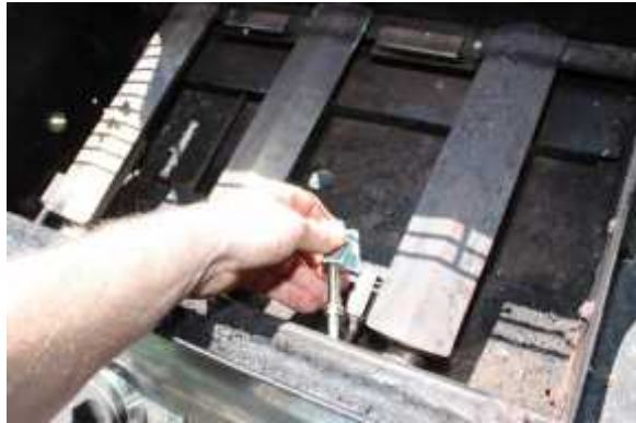
Here is a new electrode along with the old one. See Chapter 4 - Basic Grill Maintenance, Diagnostics and Trouble Shooting.
