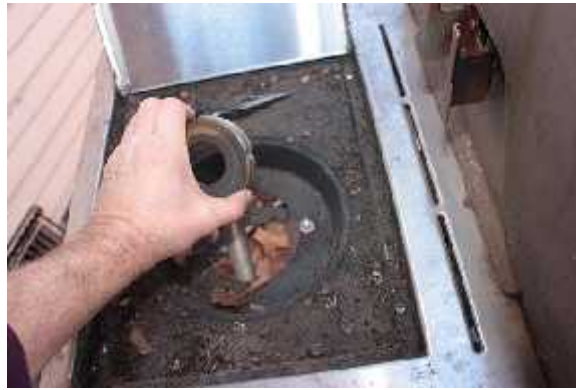
Remove side burners
